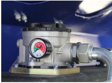
Fig 2.1. Filter Housing with Pressure Gauge
