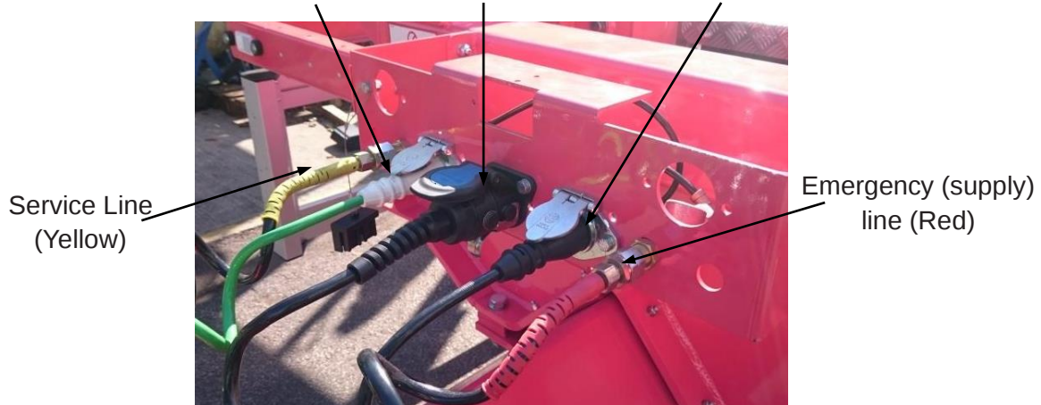
Typical Couplings (24N/24S electrical connections and "C" type pneumatic connections)
