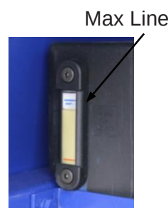
Fig 7.4 Hydraulic Tank Site Gauge
