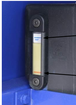
Hydraulic Tank Site Gauge
