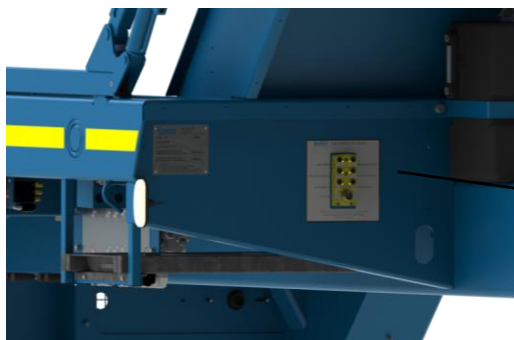
Location of Body Warning Light Module
