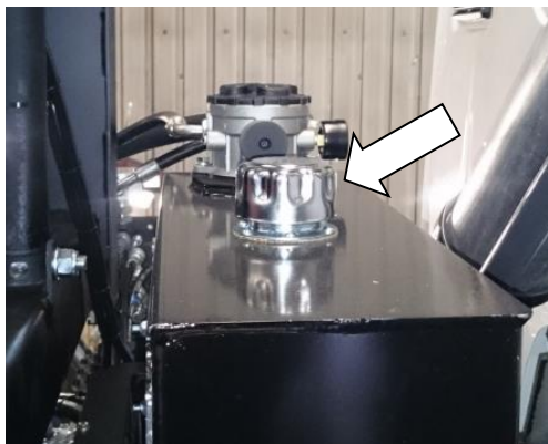
Fig. 1.2 Tank Filler Cap
