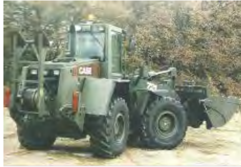
An Ulrich Simplex bucket and H 10000 winch fitted to a tractor loader
