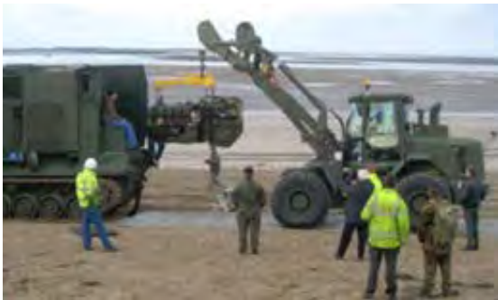
Hoist with 3 tonne tank engine Buckets and other attachments were fitted to tanks
