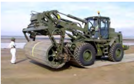
Tractor with track laying equipment
